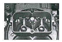
Throttle Valve-is a butterfly valve located in the air horn when it's closed it restricts air flow into the engine.
